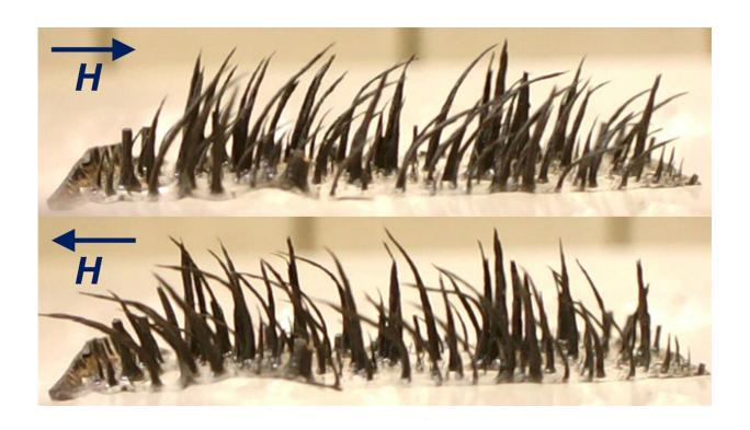
Bending of NdFeB-based magnetic cilia magnetized pointing up in horizontal magnetic fields. Credit: Matthew R. Clary.
