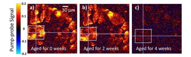
Images taken with a pump-probe microscope show how the paint samples fared over the course of the aging process. Areas that were unchanged are shown in blue, and areas where the cadmium sulfide has broken down are shown in red. Changes that were imperceptible to the eye were undeniable in the laser signal by as early as week one. Credit: Yue Zhou, Warren lab, Duke University.
