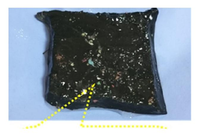
Microplastic adsorption on hydrogel and fluorescent-tagged microplastic detection via spectroscopy. Credit: Soumi Dutta
