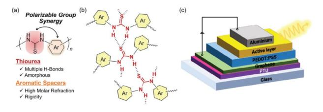
a) Molecular design of poly(thiourea)s (PTUs) with polarizable group synergy, b) plausible schematic representation of disordered (various conformational) H-bonding networks between the PTU chains enabling polarizable supramolecular networks, and c) schematic representation of the architecture of light-emitting electrochemical cells. Credit: Kenichi Oyaizu from Waseda University
