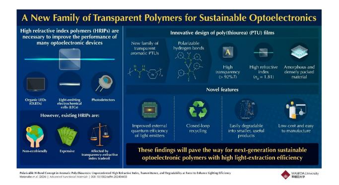
A new family of polymers based on poly(thiourea)s not only offers high transparency and high refractive index but can also be synthesized, processed, and ultimately recycled at a low cost, likely paving the way to the next generation of optoelectronic devices. Credit: Kenichi Oyaizu from Waseda University
