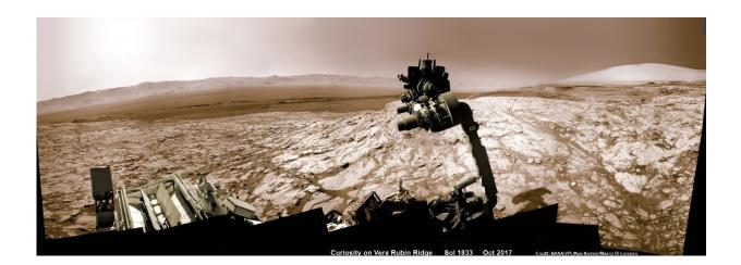
NASA's Curiosity rover raised robotic arm with drill pointed skyward while exploring Vera Rubin Ridge at the base of Mount Sharp inside Gale Crater—backdropped by distant crater rim. This navcam camera mosaic was stitched from raw images taken on Sol 1833, Oct. 2, 2017, and colorized. Credit: NASA/JPL/Ken Kremer/kenkremer.com/Marco Di Lorenzo
