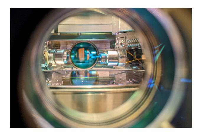
View of the optical resonator through the window of the ultrahigh vacuum chamber. Credit: Philipp Kunkel.
