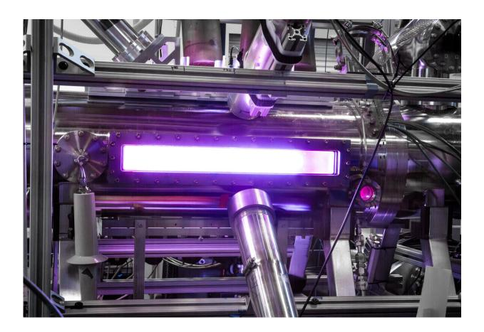
A bright flash of light from a FuZE (Fusion Z-pinch Experiment) plasma. Credit: Zap Energy
