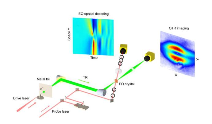
Relativistic electron bunches were generated via the incidence of a high power laser onto a gas jet. The TR radiation emitted when electron passing through a metal foil was imaged to an EO crystal. OTR imaging and EO spatial decoding were conducted simultaneously to achieve the electron spatial-temporal profile in a single shot. Credit: Kai Huang, Zhan Jin, Nobuhiko Nakanii, Tomonao Hosokai, and Masaki Kando
