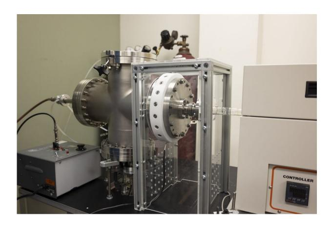
Remote plasma vapor deposition instrument designed by Fanchini Lab. Credit: Mitch Zimmer/Western Science
