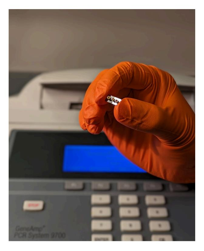
The nanopore optofluidic chip used in the new diagnostic system, with a PCR thermocycler in the background for comparison. The new system could easily fit
