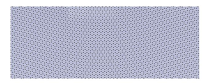
Electron microscopy image of a photonic crystal. The diameter of the triangular holes is 300 nanometers. The curvature of the crystal array stops the light waves in the crystal from moving. Credit: AMOLF
