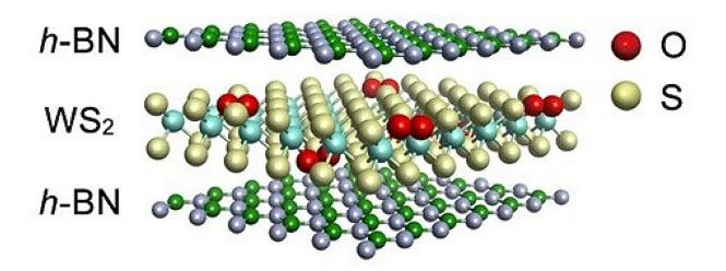
The structure of  $WS_2$  crystal monolayer, including oxygen molecules (red) adsorbed at defects, encapsulated within layers of hexagonal boron nitride. Credit: *Advanced Science* (2024). DOI: 10.1002/advs.202310197
