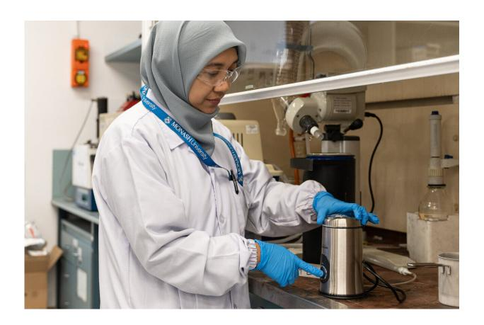
Scrap tire chips were frozen with liquid nitrogen and ground using a coffee grinder, blended with plastics and placed in a furnace at 600°C. Credit: Monash University
