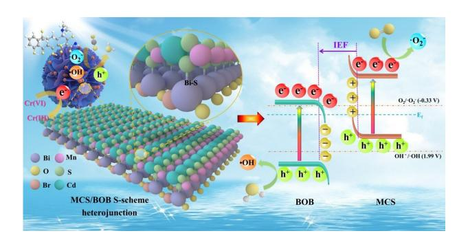
Schematic diagram of photocatalytic water decontamination mechanism. Credit: Shijie, Li et al.
