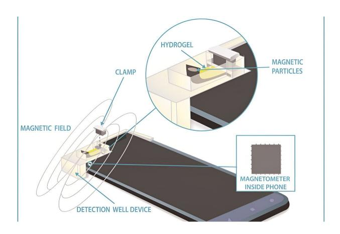
Illustration shows how a smartphone magnetometer can measure a host of biomedical properties in liquid samples using a magnetized hydrogel. Credit: K. Dill/NIST
