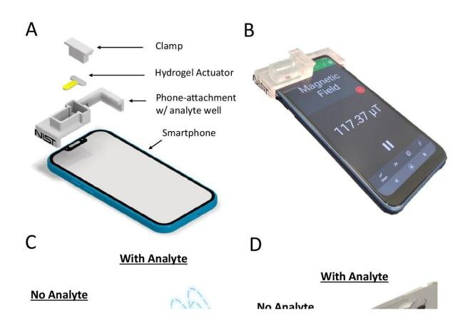
Proof-of-concept design for magnetometer-based smartphone sensing. A
