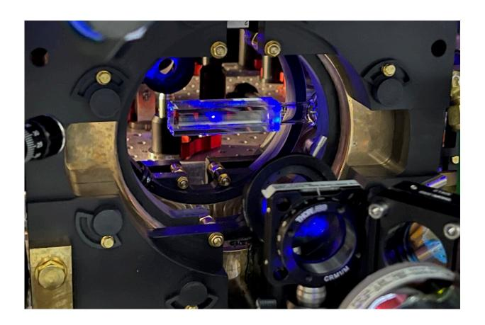
Picture of the glass cell with the strontium gas cloud in the middle. Credit: ICFO
