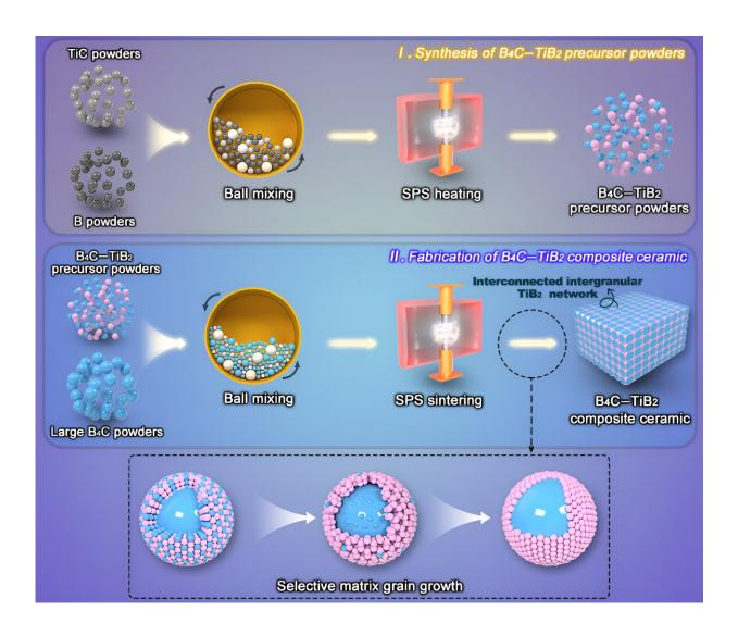
First,  $(B_4C-TiB_2)$  precursor powders were designed and synthesized from boronizing process of TiC. Second, the precursor powders were mixed with commercial B<sub>4</sub>C powders, and the B<sub>4</sub>C-TiB<sub>2</sub> composite ceramics were
