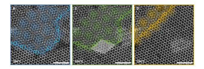
Annular dark field scanning electron microscopy images of a bilayer interface after heat pulses at 500° (left), 600° (middle) and 700° (right). Dashed colored lines mark the positions of the interface as it is displaced with heating. Credit: The Grainger College of Engineering at University of Illinois Urbana-Champaign
