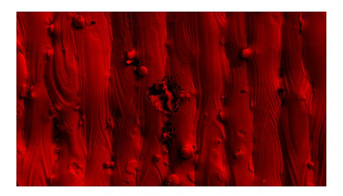
A photo taken by a scanning electron microscope shows a pit at the surface of an additively manufactured (3D-printed) stainless steel part. Credit: Thomas Voisin.
