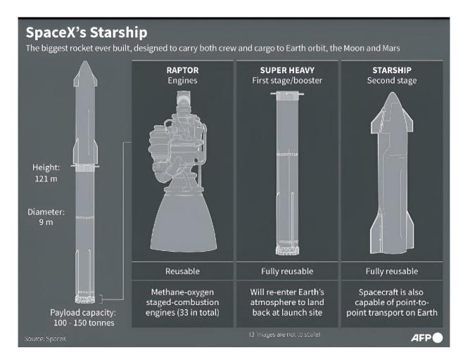
Graphic on SpaceX's Starship launch vehicle, the biggest rocket ever built.
