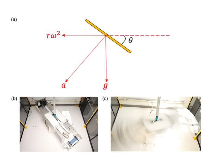
(a) Illustration of the net force experienced during crystallization, which is the vector sum of the gravitational force and the centrifugal force. (b) Photographs
