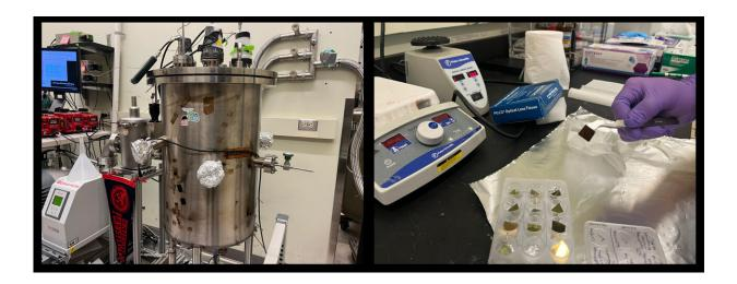
Nicknamed "Defiant," the Fakhraai Group's custom-made ultra-high vacuum chamber (left) is used for physical vapor deposition of organic glasses. Image on the right is of 180 nm thick stable glass films of N,N'-bis(3-methylphenyl)-N,N'-diphenylbenzidine, deposited on polydimethylsiloxane-coated silicon wafer. Credit: Nathi Magubane
