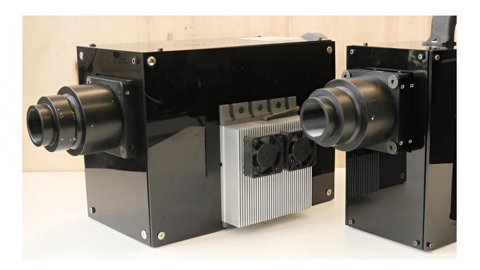
Scientists at EPFL have published a guide to building an add-on that turns a standard optical microscope into an instrument capable of producing super resolution, 3D images of cells, organoids, and embryos. Credit: Ecole Polytechnique Federale de Lausanne
