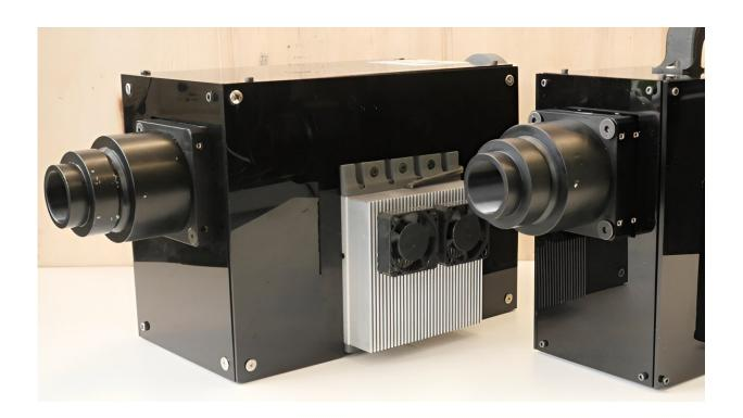
Scientists at EPFL have published a guide to building an add-on that turns a standard optical microscope into an instrument capable of producing super resolution, 3D images of cells, organoids, and embryos. Credit: Ecole Polytechnique Federale de Lausanne
