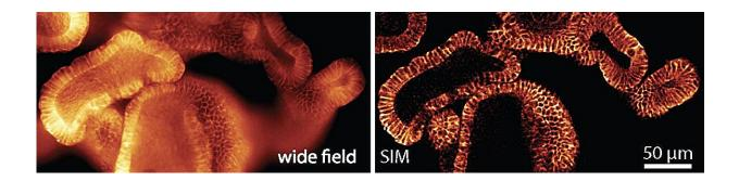
Illustration of the optical sectioning effect when using the openSIM. On the wide field image, out of focus light is noticeable in the image; on the openSIM image, only the part of the sample directly in focus is visible. Sample: fixed mouse intestinal organoids labeled for E-cadherin. Credit: LBNI
