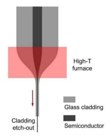
A schematic diagram of the semiconductor fiber manufacturing method developed by the NTU research team. Credit: Nanyang Technological University
