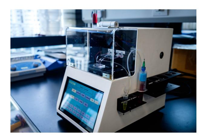
Prototype of the ExoArc system, which allows for a one-step automated isolation of high-quality blood plasma useful for diagnostics and precision medicine. Credit: Nanyang Technological University
