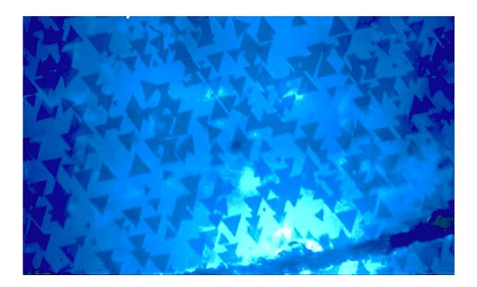
False-color optical image of the MoS2 crystals grown at a high temperature and low flow rate, where the largest average crystal size is obtained among the tested growth conditions. Credit: Jun Lou/Rice University
