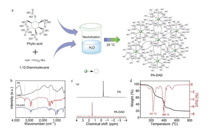
(a) Schematic diagram for the prepared processing of PA-DAD, (b) FTIR spectra of DAD, PA and PA-DAD, (c) 31P NMR curve of PA-DAD and PA, (d) TG curves of PA-DAD. Credit: *Emergency Management Science and Technology* (2023). DOI: 10.48130/EMST-2023-0021
