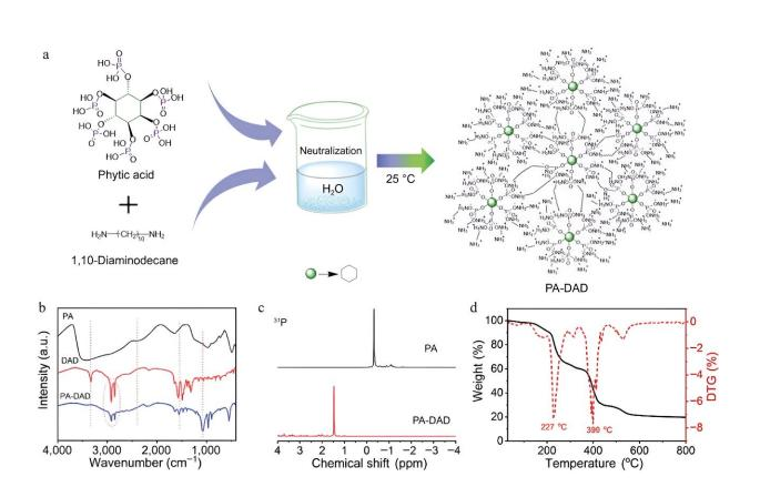
(a) Schematic diagram for the prepared processing of PA-DAD, (b) FTIR spectra of DAD, PA and PA-DAD, (c) 31P NMR curve of PA-DAD and PA, (d) TG curves of PA-DAD. Credit: *Emergency Management Science and Technology* (2023). DOI: 10.48130/EMST-2023-0021
