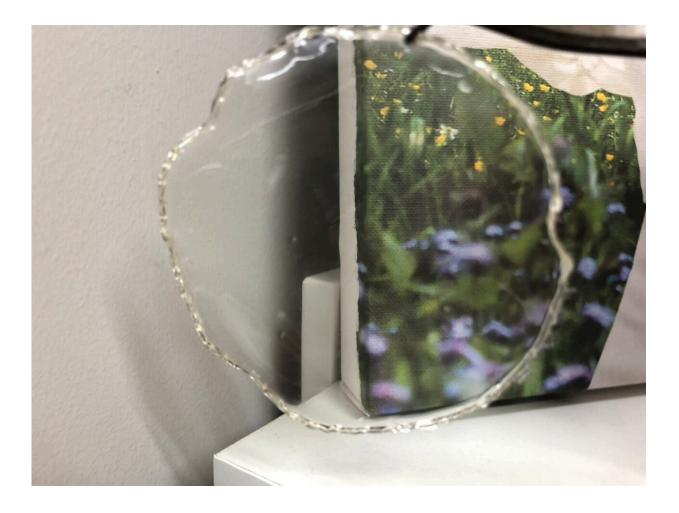
A transparent film made from the new recyclable polymer developed in this study. Credit: Feng Li
