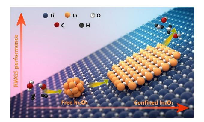
Confinement-induced indium oxide nanolayers formed on  $TiO_2$  for enhanced  $CO_2$  hydrogenation reaction. Credit: Wang Jianyang
