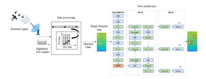
Simplified block diagram of a generic pulse-doppler radar system and consequent digital processing, with the introduction of YOLO-based moving target detector after the matched filter. Credit: *IET Radar, Sonar & Navigation* (2024). DOI: 10.1049/rsn2.12547
