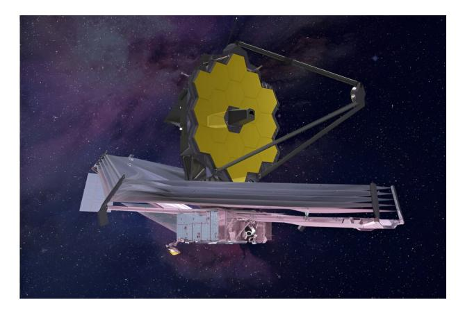
The James Webb Telescope — the largest and most powerful device of its kind ever launched into space — uses a 6.5-metre primary mirror, made of 18 hexagonal mirrors, coated with a plating of gold to produce some of the earliest images of the universe. Credit: NASA
