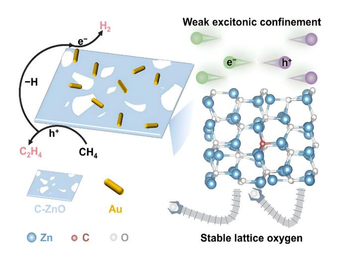
A stoichiometric photocatalytic methane conversion via 2CH<sub>4</sub> = C<sub>2</sub>H<sub>4</sub> + 2H<sub>2</sub> is achieved over C-ZnO/Au due to reduced excitonic binding energy and stable lattice oxygen. Credit: Science China Press
