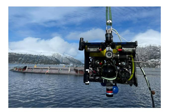
Does this robot disturb penned fish? It is equipped with an echo sounder and cameras that enable it to observe how the fish around it respond to its movements. Here we see it being lowered into the water at a location offshore Kristiansund. Credit: SINTEF
