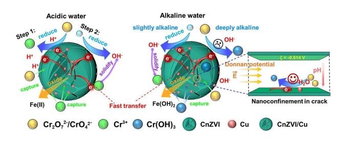
Schematic illustration of Cr(VI) removal mechanism by CnZVI/Cu at acidic/alkaline conditions. Credit: Li Sijia
