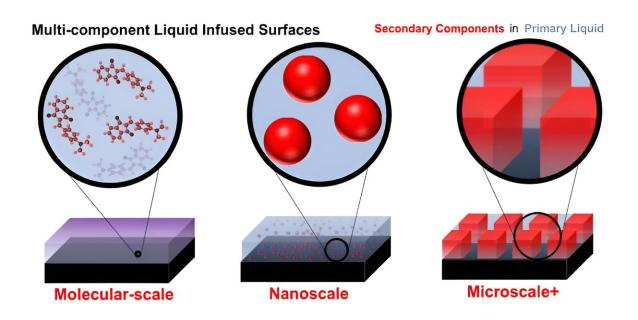
Adding a secondary component to a liquid coating results in new and synergistic properties. Credit: Caitlin Howell, University of Maine, U.S.
