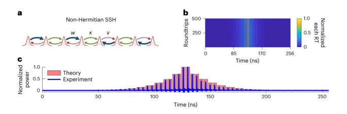
Nonlinearity-driven NHSE in a topological mode-locked laser. a, Schematic representation of the NH-SSH domain wall implemented in our mode-locked laser's synthetic lattice. b, Heat map of our mode-locked laser's output over 500 roundtrips. The pulses are broadened for visibility. c, Mode-locked pulse pattern in our topological mode-locked laser. Credit: *Nature Physics* (2024). DOI: 10.1038/s41567-024-02420-4
