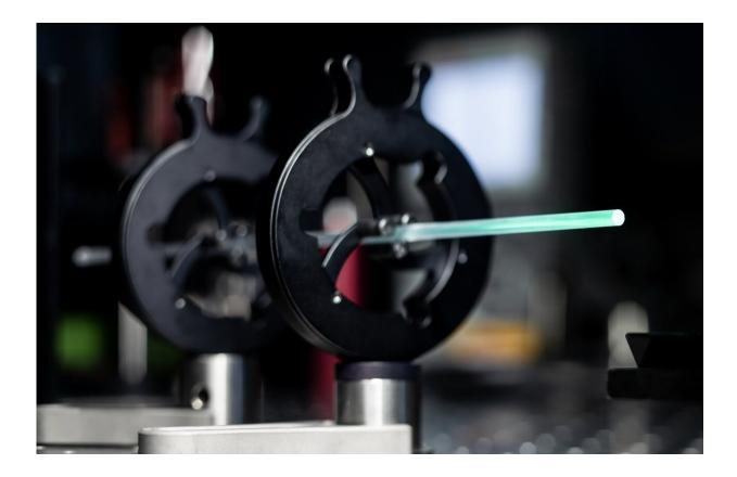
Ytterbium-doped glass rod excited by laser. Credit: Fraunhofer IOF
