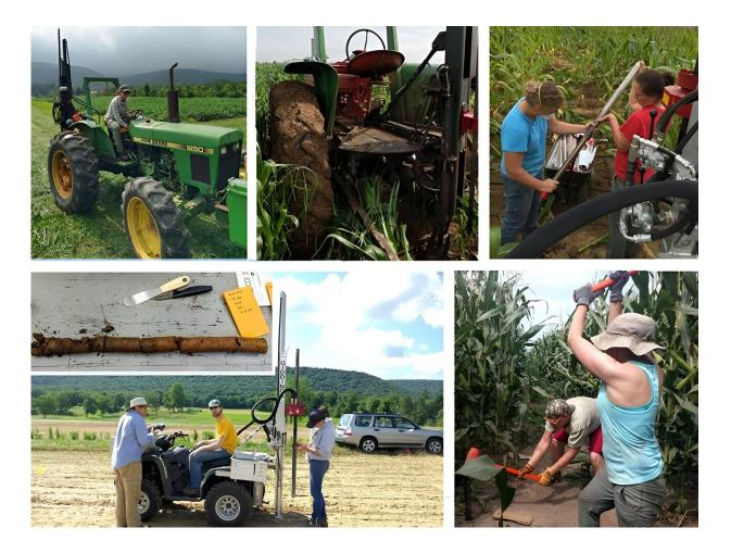
Developing the new method took six years and involved the collection and analysis of more than 2,000 soil core samples at four research sites across the country. These images show researchers getting core samples using a device mounted on the back of a tractor and an ATV, and the old-fashioned way with a tube and sledgehammer. Credit: Penn State
