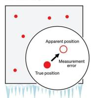
The apparent but incorrect position of the quantum dot misguides the placement of a photonic component, such as a circular grating, resulting in misalignment.
