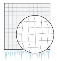
Measurement errors result from these optical imperfections, causing the apparent position of a quantum dot in a microscope image to differ from its true position.
