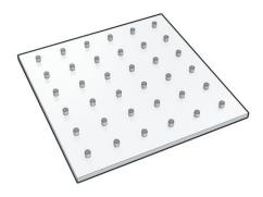
The traceable spacing of the pillar array enables an accurate calibration of magnification and a correction of position errors due to image distortion.
