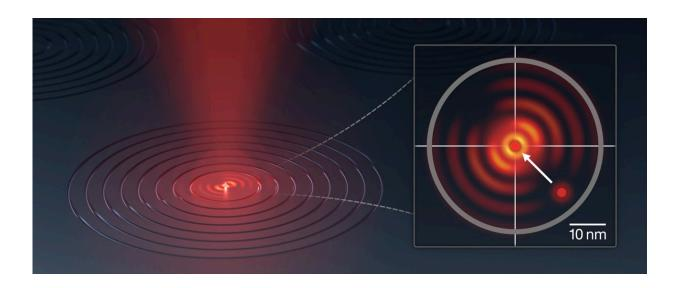
Accurate alignment of quantum dots with photonic components is critical for extracting the radiation emitted by the dots. In this illustration, a quantum dot centered in the optical "hotspot" of a circular grating (center dot in the inset) emits more light than a dot that is misaligned (off-center dot in the inset). Credit: S. Kelley/NIST
