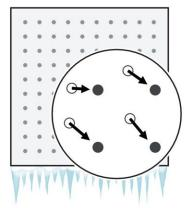
Illustration showing how traceable calibration of an optical microscope can correct for instrument imperfections that would otherwise result in misalignment of quantum dots with photonic components. Credit: S. Kelley/NIST
