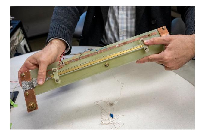
An experimental board containing a superconducting tape-shaped HTS material called Bi-2223 and a controlled heater is used to test the thermal runaway-based concept of magnet protection. Credit: Marilyn Sargent/Berkeley Lab
