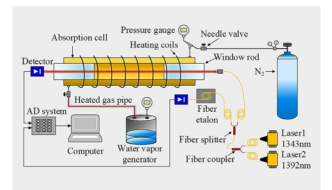
Concentration-Independent Pressure Sensing Method Developed for High-Temperature Combustion Diagnostics. Credit: Wang Ruifeng
