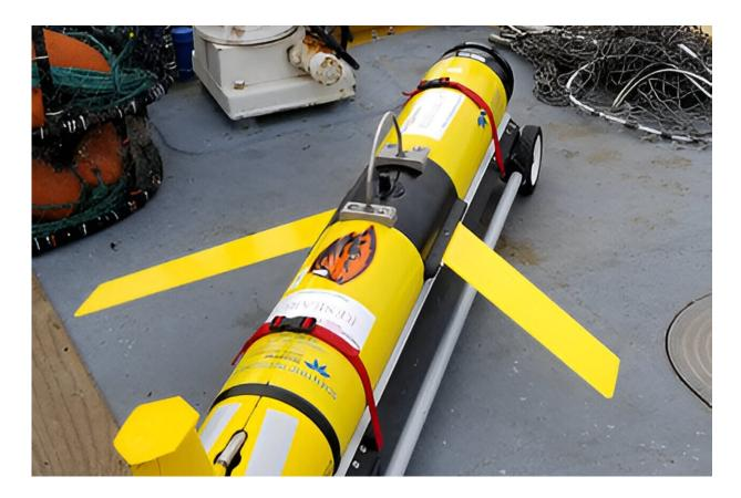
In late August, OSU's Jack Barth and his colleagues deployed a glider that traversed Oregon's near-shore waters from Astoria to Coos Bay and measured the oxygen levels through the water column, and beamed the data back to OSU computers. Credit: Jack Barth.
