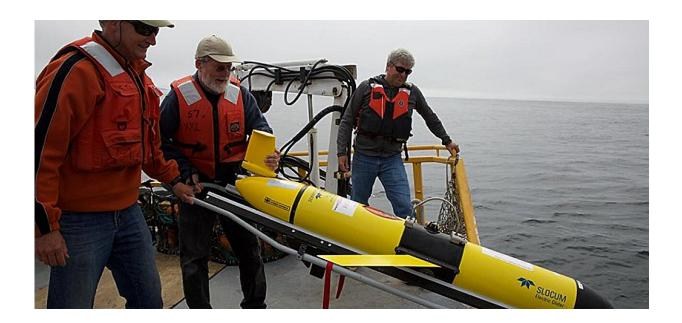
In late August, OSU's Jack Barth and his colleagues deployed a glider that traversed Oregon's near-shore waters from Astoria to Coos Bay and measured the oxygen levels through the water column, and beamed the data back to OSU computers. Credit: Jack Barth.
