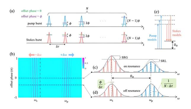
Fig. 1. Working principle of Stimulated Raman Scattering driven by femtosecond-pulse burst. Credit: *Light: Science & Applications* (2024). DOI: 10.1038/s41377-023-01367-0
