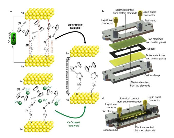
Catalysis of a click reaction in a microfluidic cell. Credit: *Nature Communications* (2024). DOI: 10.1038/s41467-024-44716-2
