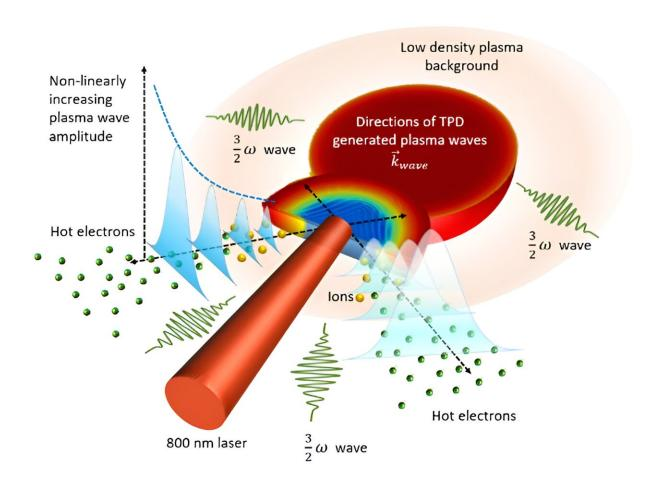
Laser beam incident on the structured droplet sets up plasma waves (blue pulses) that accelerates electrons (green solid spheres) to megaelectronvolt energies. Credit: Adapted from *Communications Physics* (2024). DOI: 10.1038/s42005-024-01550-8
