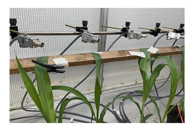
The EPG system at work in the laboratory: electrodes are connected to insects on corn plants. Credit: Nathalie Maluta
