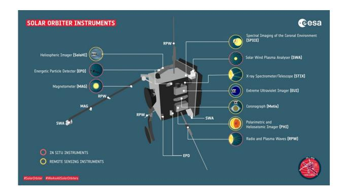
Solar Orbiter's suite of ten science instruments that will study the Sun. There are two types: in situ and remote sensing. The in situ instruments measure the conditions around the spacecraft itself. The remote-sensing instruments measure what is happening at large distances away. Together, both sets of data can be used to piece together a more complete picture of what is happening in the Sun's corona and the solar wind. Credit: European Space Agency
