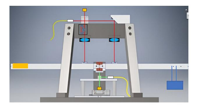
Scheme of the balanceprototype including the opticalread-out and the aluminumsuspended sample (in blue) and the brass counterweight (in orange). Credit: *The European Physical Journal Plus* (2024). DOI: 10.1140/epjp/s13360-024-04920-x
