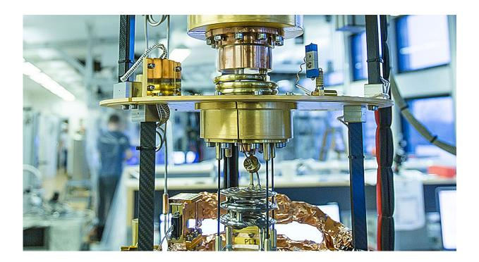
The biggest challenge in the development of the quantum computer consists of the magnetic and electrical noise that disturbs the quantum effect, and therefore the processor QPU (Quantum Processing Unit) is cooled down to the lowest possible temperature just above the absolute zero point of -273 degrees. This happens in the cryostat, which can be seen in the picture. The processor is located at the bottom of the cryostat. Credit: Ola J. Joensen, NBI
