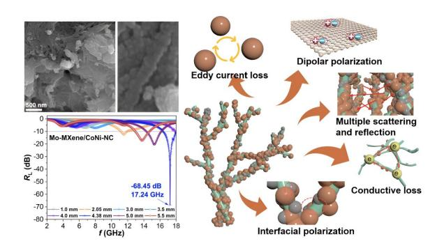
The zigzag-like Mo-MXene/CoNi-NC material exhibits excellent electromagnetic wave absorption properties due to its perfect balance between dielectric loss and magnetic loss. The material can be interpreted through SEM, 2D R<sub>L</sub>, and mechanistic analysis. Credit: Journal of Advanced Ceramics, Tsinghua University Press
